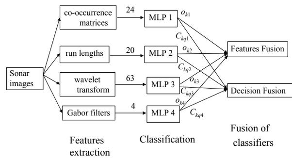
Figure 5. Architecture of fusion.
