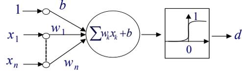
Figure 4. Artificial neuron structure.
